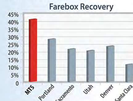
Percent of total operating costs paid for directly by passengers with their fare. Farebox recovery is improved by: 1) increasing ridership; 2) reducing costs; and/or 3) increasing fares.
