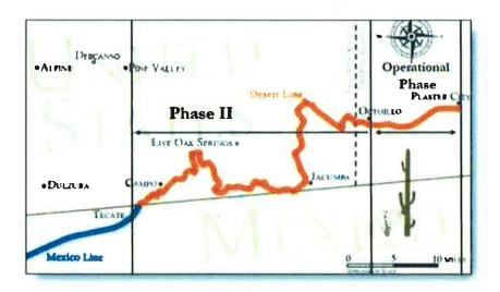
The operational phase includes 9.5 miles of track from Coyote Wells (milepost 120.09) to Plaster City (milepost 129.61) and involves repairing 11 bridges as well as the track, ties, and ballast in order to get this portion of the line to a FRA class III standard. This portion of class III track will connect the intermodal facility at Coyote wells
