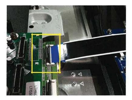
3. Verify that the ribbon is placed all the way in and properly into the slots.
