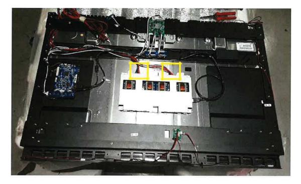
3. Make sure that both cables are secure, you may want to try disconnecting and reconnecting the cables.
