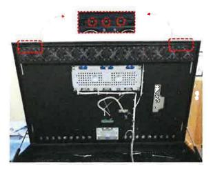
3. Separate LCD module from the front glass.
