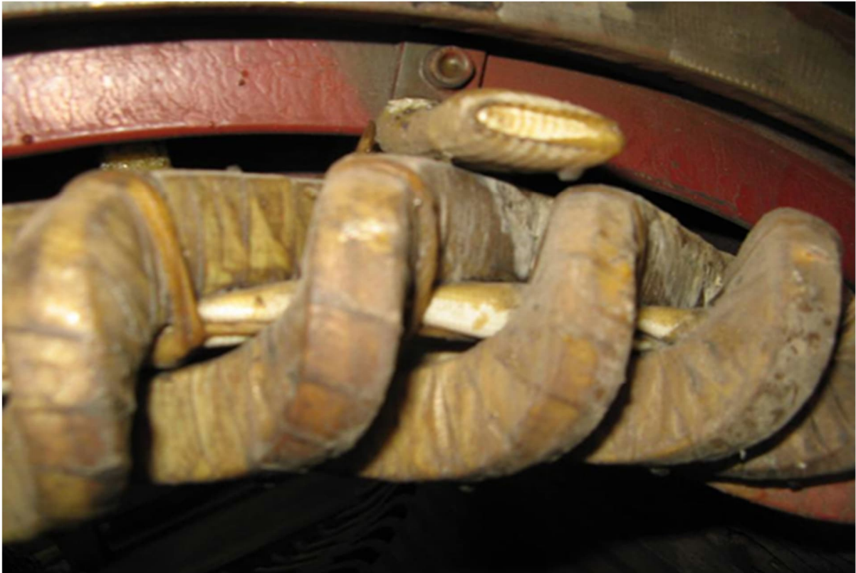
Figure 4 - Motor windings rewound by independent shop
