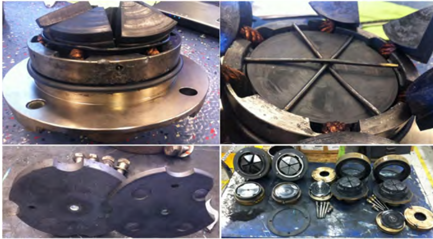
Figure 1 - Damaged Grounding Contacts
