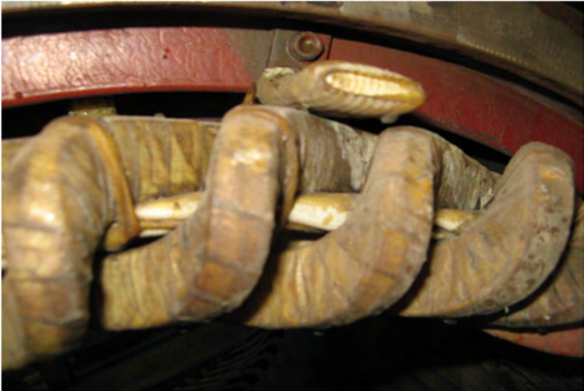
Figure 4 - Motor windings rewound by independent shop
