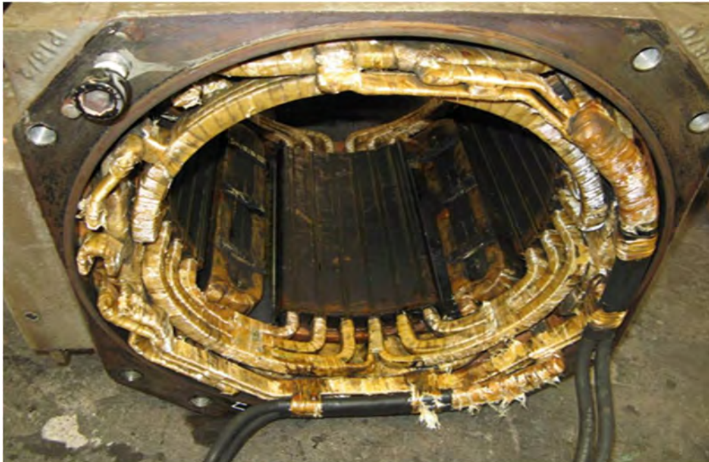
Figure 3 - Motor cleaned with improper chemicals
