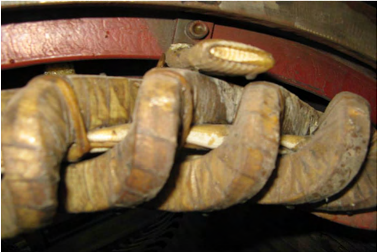
Figure 4 - Motor windings rewound by independent shop
