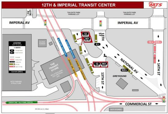
Figure 1. Current Layout of 12th and Imperial Transit Center
