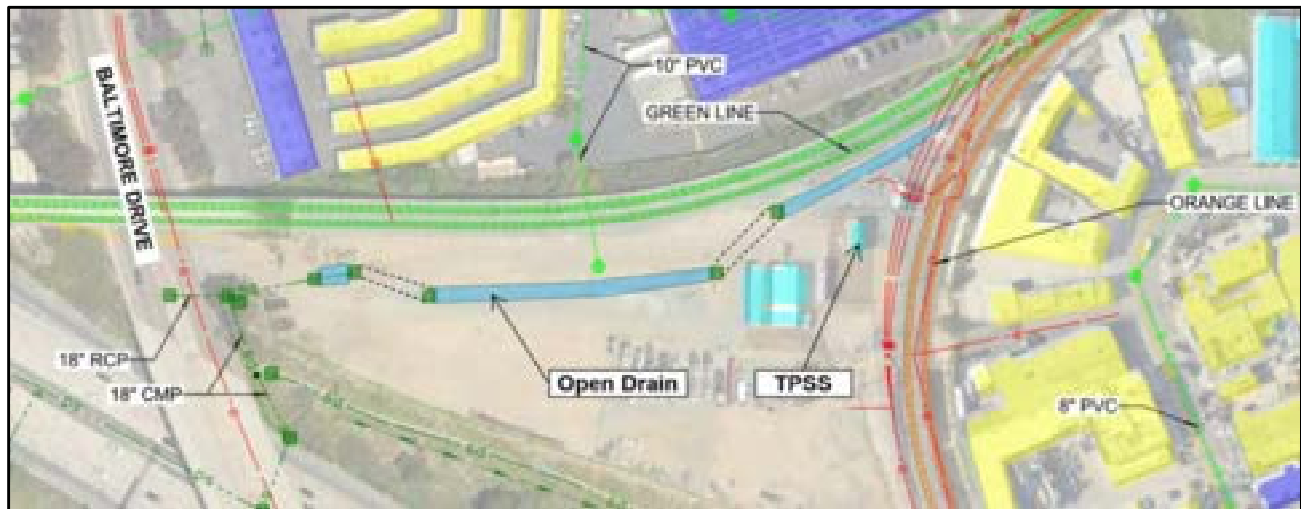
Figure 2-8 Open Channel Drainage and Site Utilities
