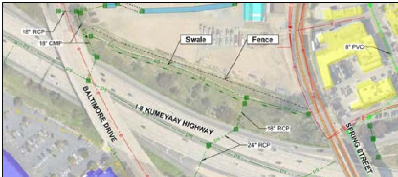
Figure 2-11 Caltrans Swale and Fence
