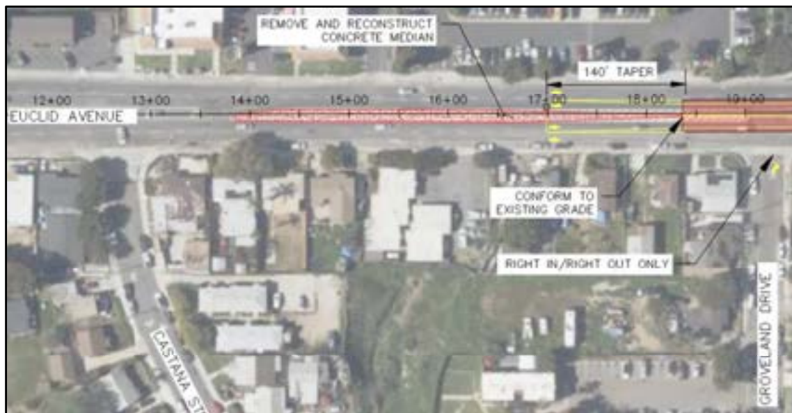
Figure 3-22: South End Lane Taper Transition
