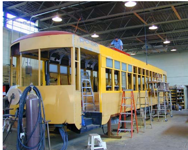
Figure 4-15: Replica Birney Streetcar Assembly Line
