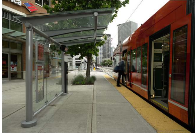
Figure 4-12: Low-Floor Boarding in Seattle
