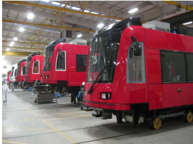
Figure 4-13: Siemens SD8 Modern Streetcar Assembly Line
