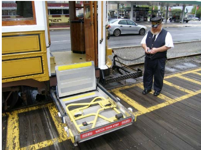
Figure 3-3: On-Car Lift on Historic Streetcar
