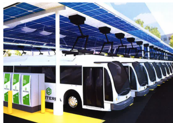
Exhibit 11: Depot Charging with Inverted Pantographs
