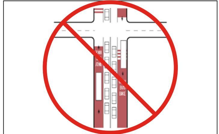
Figure 2-15 Shared Transit and Bike Lanes are Not Recommended Source: NACTO Transit Street Design Guide
