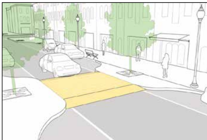
Figure 2-11 Speed Table Source: NACTO Urban Street Design Guide
