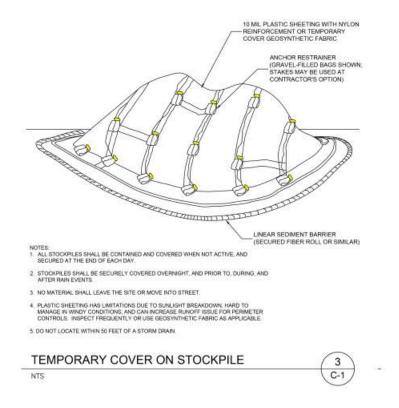
Figure 1. Stockpile Management for Temporary Storage of Solids and Debris
